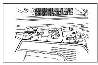
The surge tank is located on the driver side of the engine compartment. See *Engine Compartment Overview on page 5-12* for more information on location.
